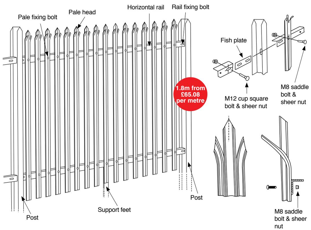
We stock triple pointed pale tops in 'D' 3mm and 'W' 2mm thickness profile sections. Our metre runs include all fixings, pales, posts and rails in galvanised finish. Available for 1.8, 2.0, 2.1, 2.4 and 3m fence heights.
