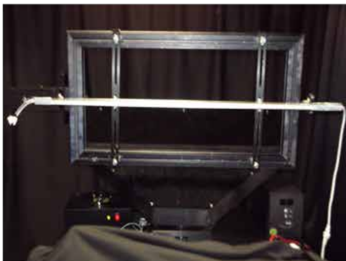
PHOTO 1: LUMINAIRE ON GONIOMETER MOUNT
