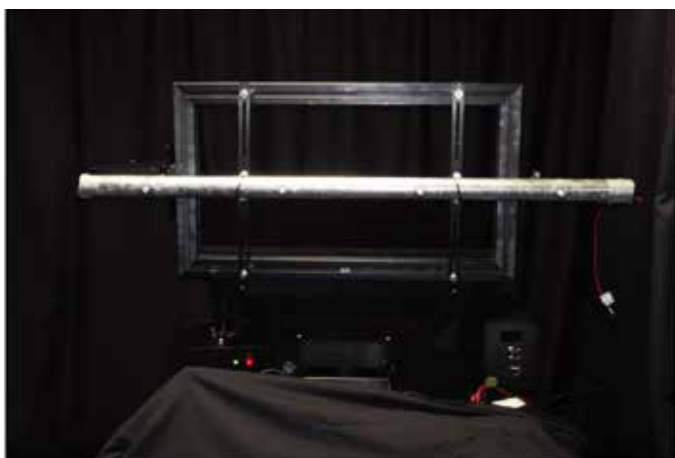
PHOTO 1: LUMINAIRE ON GONIOMETER MOUNT
