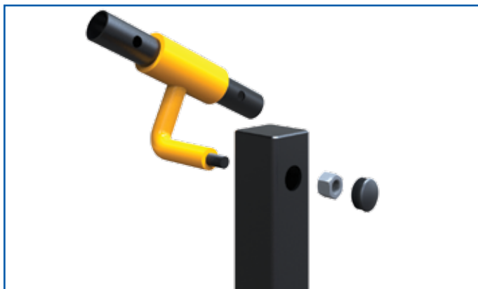
Pre-drill steel RHS post and then bolt handrail bracket from the inside of the RHS section. Use a plastic cap, from our 3201 range to conceal hole, see page 31.
