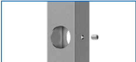
Grub screw prevents tube rotation.
