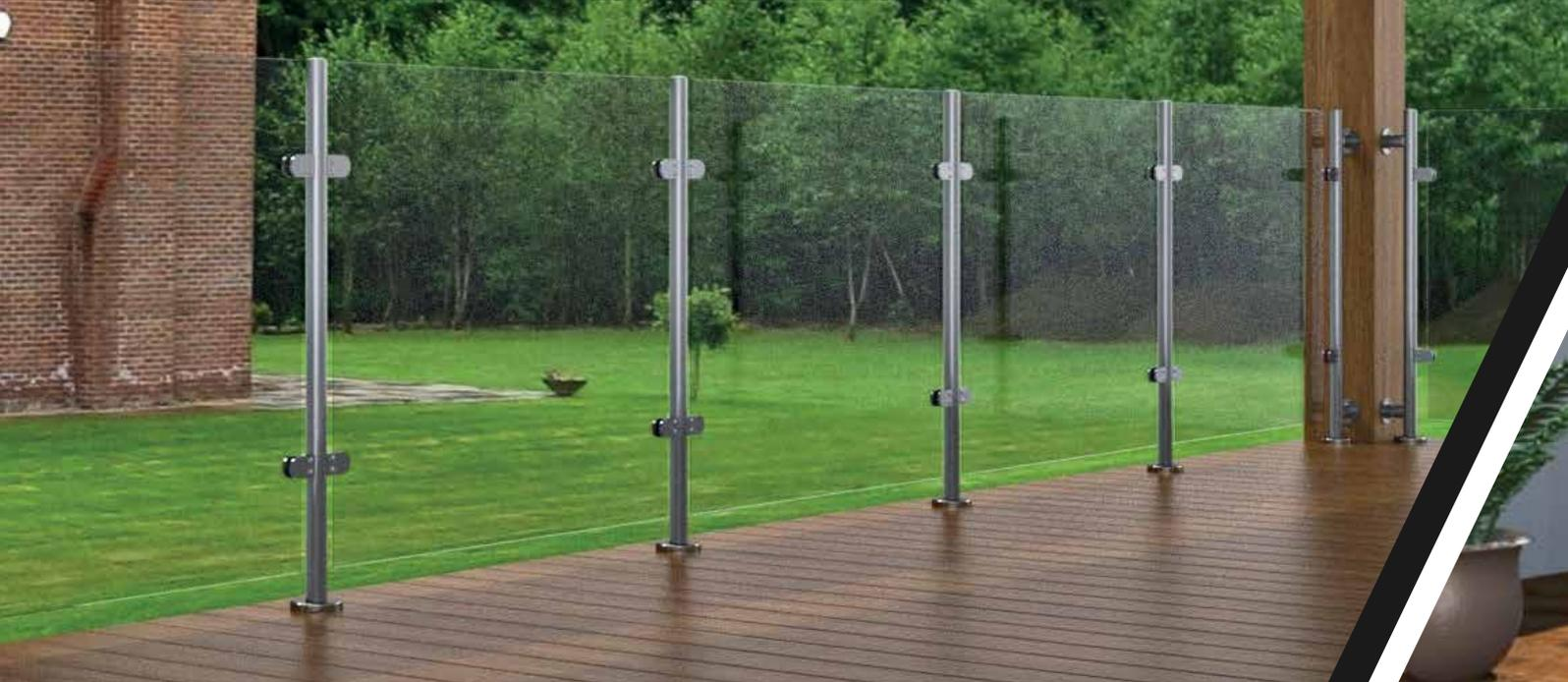
Our pre-assembled post system is designed to make life easier with a variety of spigots to meet most needs. Suitable for use with drops under 600mm without handrails. Bolt-down, concrete-in and side-fix options are available. We also stock a range of 10mm thick glass panels.
