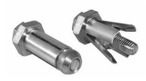
**BoxBolt** is a fully tested and approved blind fixing solution for connecting to hollow section steelwork or where access is restricted to one side only. **The BoxBolt** fixing is suitable for use with rectangular, square and even circular hollow sections.
