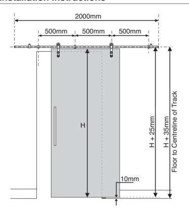
Note: Must be installed into a solid wall
