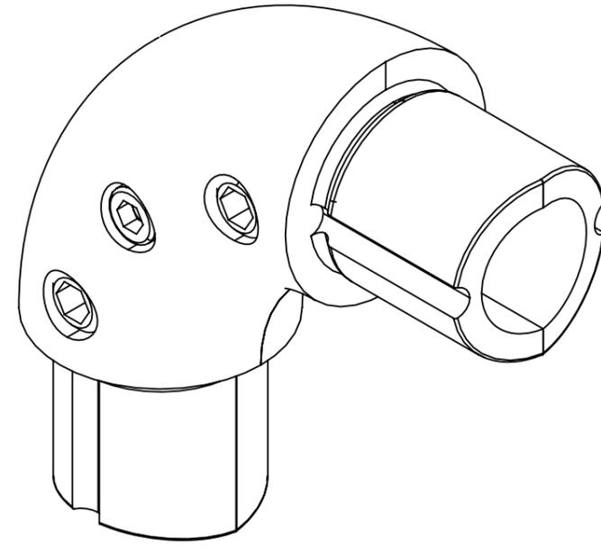
Expanding elbow for creating a smooth 90° bend in the 42.4mm o/d tube.
