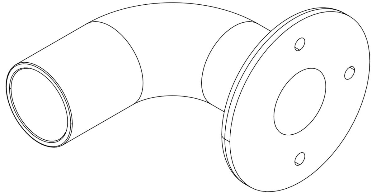
Bracket for terminating the 42.4mm o/d handrail tube back to a wall. This bracket is used in conjunction with a DDA07.
