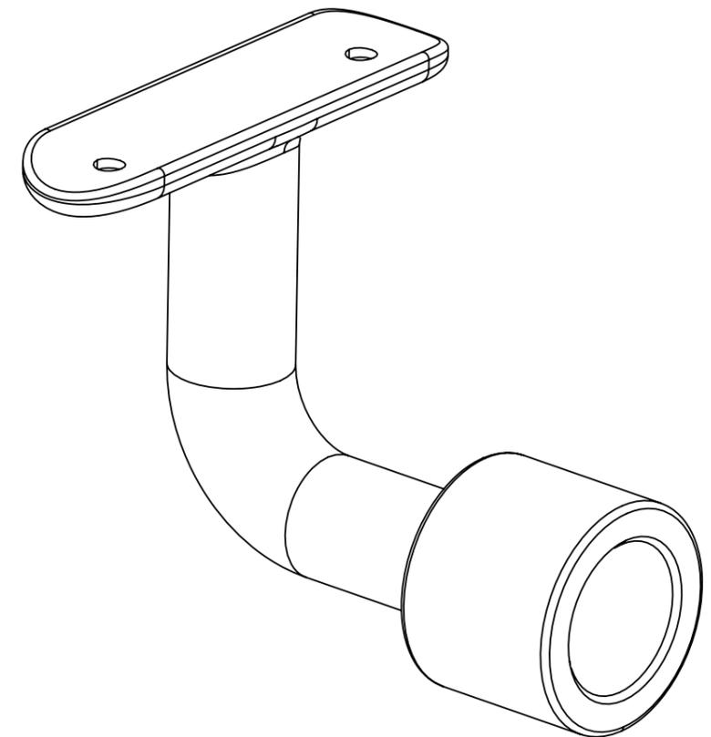
Bracket for supporting the top or middle rail tube at an upright in conjunction with a DDA01. The 42.4mm o/d tube is fixed to the DDA04 using either 2 x self tapping screws or 2 x pop rivets.
