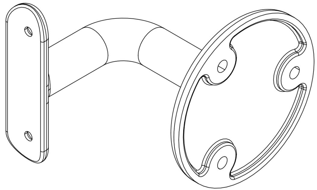
Bracket for supporting the 42.4mm o/d handrail tube to a wall.
