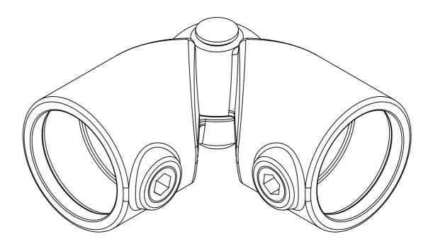
Type BC123 fitting has been designed as a variable angle inline connection, adjustablethrough 202°.
