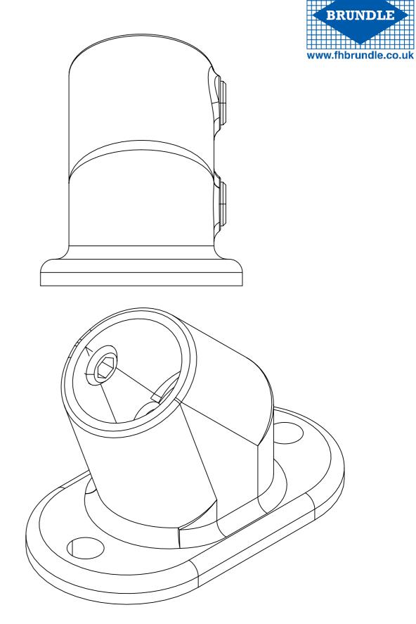
Similar to a type 151, it is used to set the upright at an angle between 30° & 45°. This fitting should only be subjected to light loads which cannot be positioned at 90° to the applied load. For greater load use a type 132 and bend the upright.
