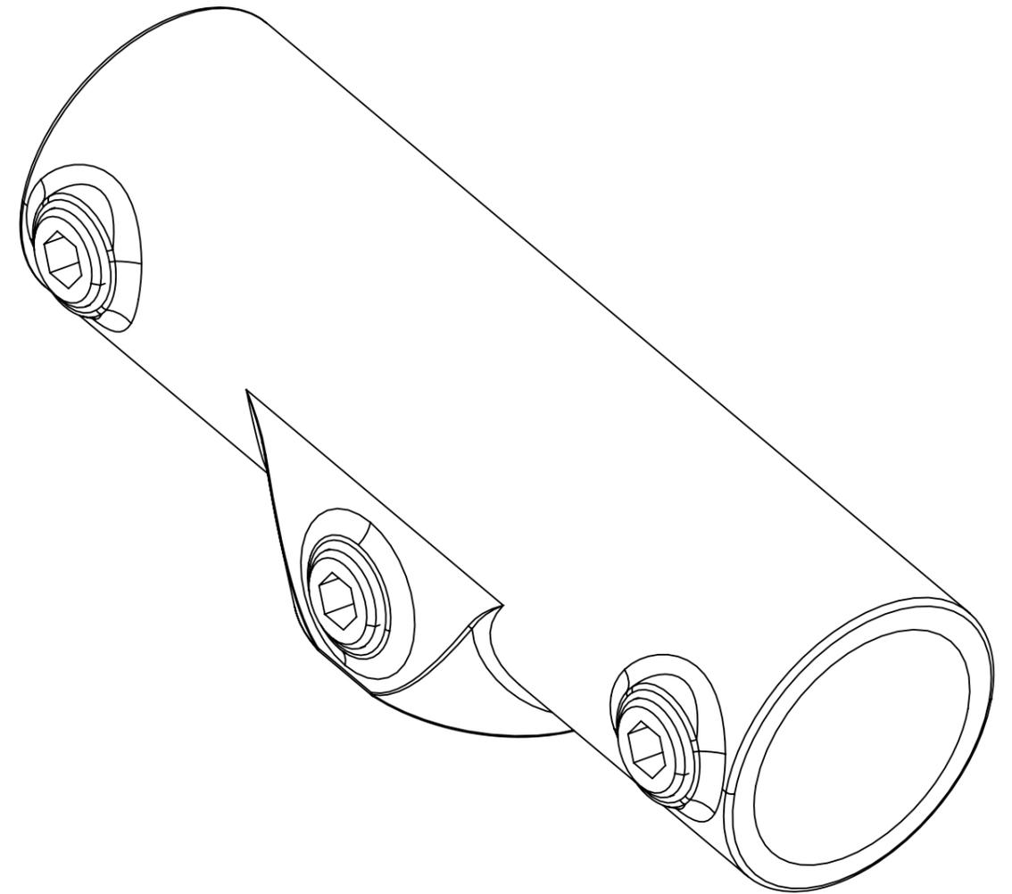
This fitting is used on Safety Railing with slopes between 11°-30° and fixes the top rail to a vertical intermediate upright.
