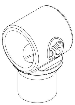
Typically used for offset variable angle sloping guardrail in conjunction with a 101 or 125 fitting.
