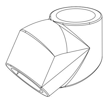
Typically used on steeper slopes or stairs as a tee connector with an angle between 30° & 60° with the upright remaining vertical. Tube cannot be joined within the fitting. Normally used in conjunction with the 130 fitting.
