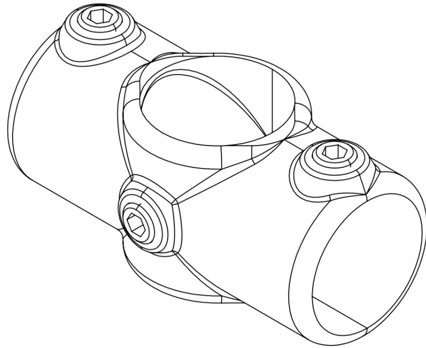
Typically used on straight and level guardrail to connect the mid rails to the upright. The upright must remain continuous with the cross rails being cut. Normally used in conjunction with the 104 fitting when building a two rail guardrail.
