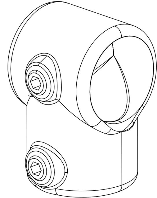
Typically used on straight and level guardrail to connect the upright to the top rail or the end or mid rail to the upright. Tubes cannot be joined inside a 101; to join tubes inside the fitting use a 104. Normally used in conjunction with the 119 fitting when building two rail guardrail.
