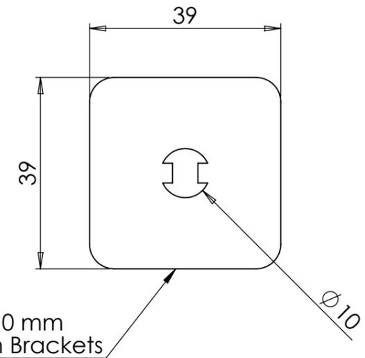
3 mm Thick EDPM Rubbers To Clamp 10 mm Thick Glass Between Brackets
