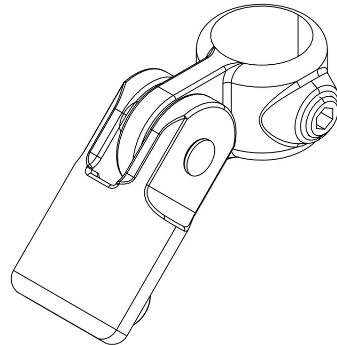
Single inline swivel connector. Typically used on sloping guardrail. This fitting combines 1 x 173M & 173F. The swivels can travel approximately 85° from the horizontal in both directions. **THIS FITTING IS NOT DESIGNED TO WITHSTAND LATERAL LOADINGS. AN ENTIRE STRUCTURE SHOULD NOT BE BUILT ONLY USING SWIVEL FITTINGS, THIS WOULD BE UNSTABLE.**
