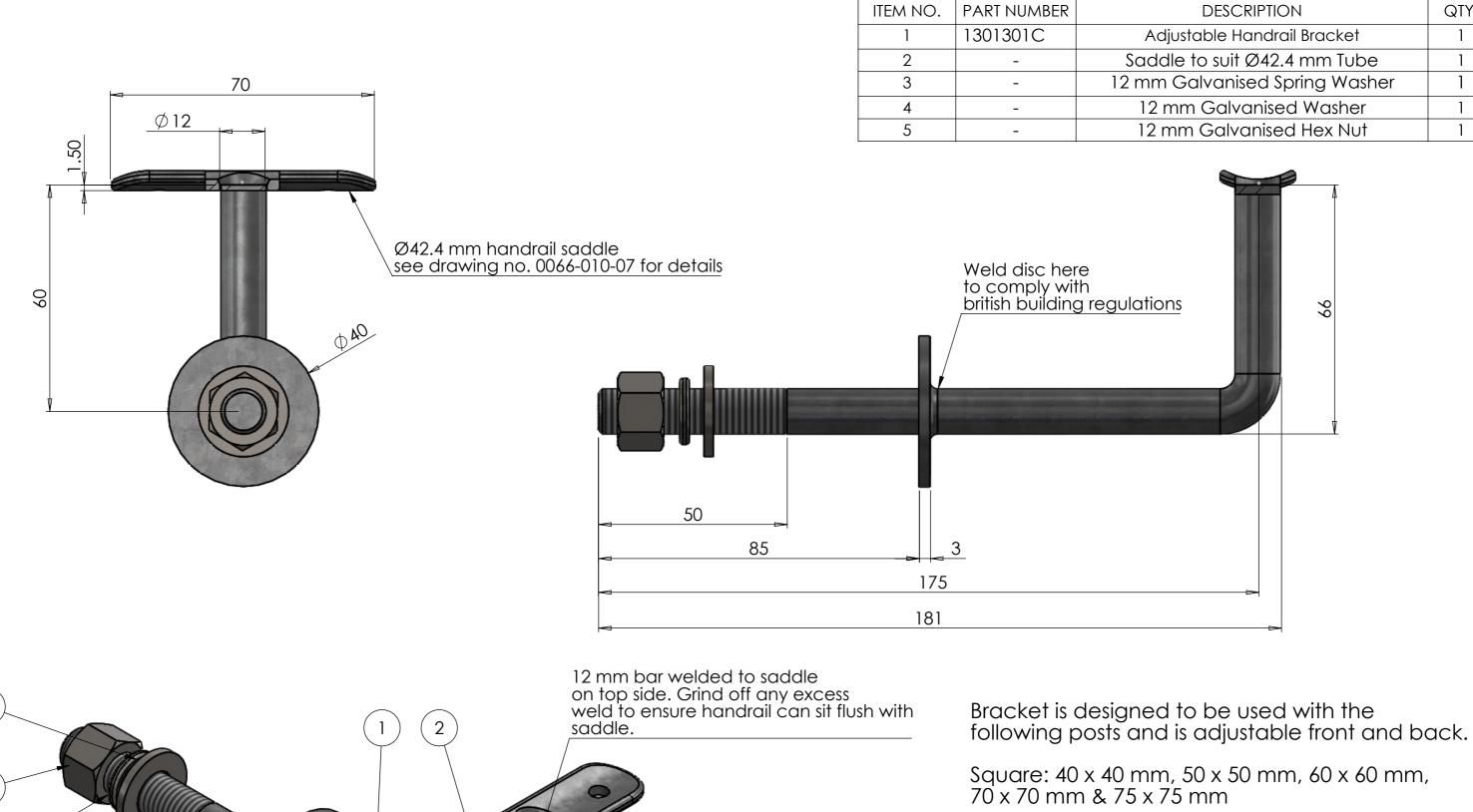
Ø40 x 3 mm Disc Welded to 12mm round bar
